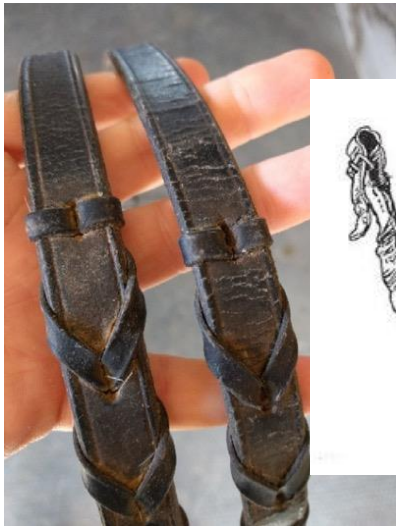
Cracked & dry Leather
